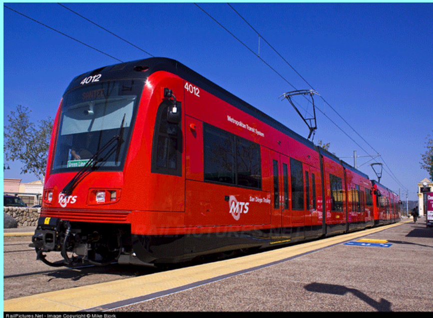
SDMTS 4012 and mate, two of the 65 Siemens S70 Ultrashort 70% Low Floor LRVs currently on the San Diego "Trolley" System!
